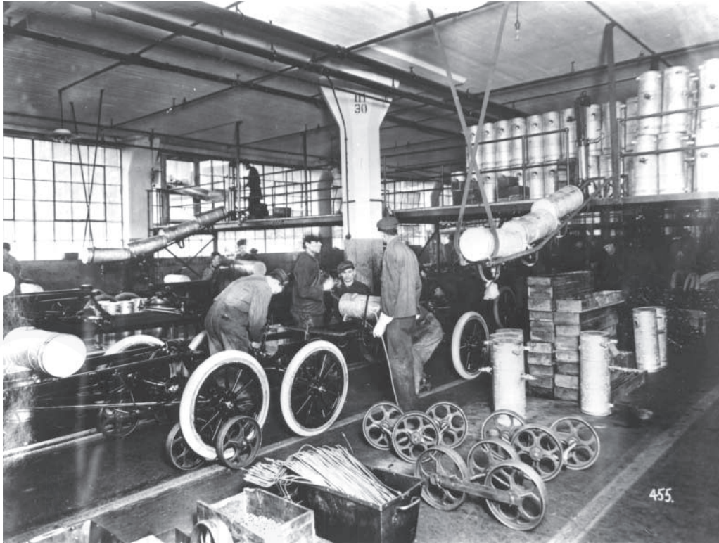
Figure 1.4 Early mass production at Ford's Highland Park plant in Detroit in 1914: the fuel tank assembly station. The chassis are moved on a track, and the cylindrical fuel tanks are supplied to the assemblers from an overhead store. The production techniques may look somewhat rudimentary by modern standards, but were innovative in their time. (Photo courtesy of Ford Motor Company Ltd.)
