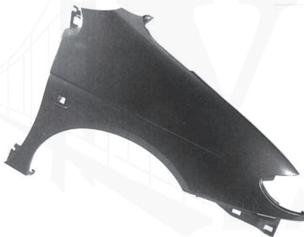
Figure 2.2 A typical plastics composite body panel
