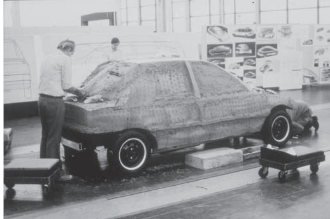
Figure 4.8 Claying up armature to hardpoints
