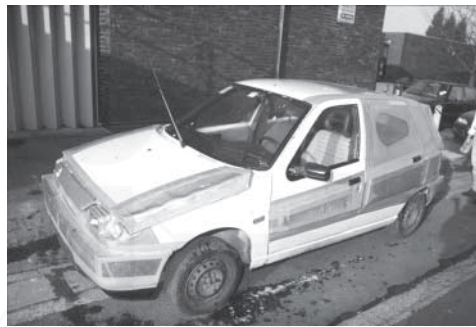
Figure 9.8 One of the camouflaged Fiat Punto prototypes used in the road trials
