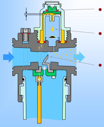
Turn the green control to adjust the oil flow restriction
