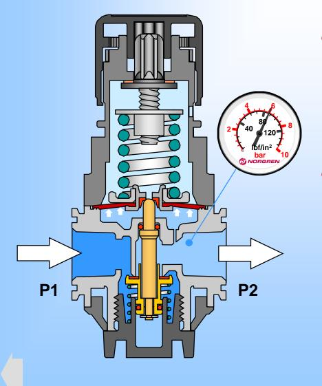
When the desired pressure is reached the force on the diaphragm will fully balance the force on the spring and the valve will close
