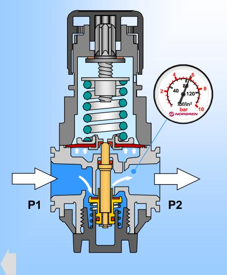
While flow is taking place the valve will be held open wide enough to keep as close to the set pressure as possible for the flow demand
