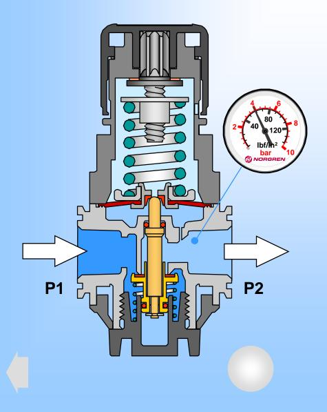
Once the desired setting has been established push down the locking adjusting knob to prevent inadvertent changes
