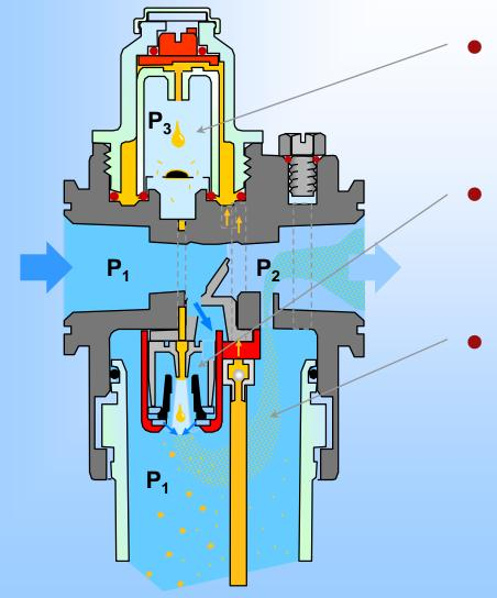
Oil drips visible through the sight dome pushed by the pressure difference between P<sub>1</sub> and P<sub>3</sub>
