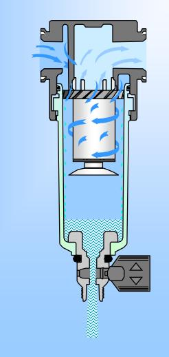
Daily visual inspection is required to ensure the water contaminant level is prevented from rising to a level where it can be drawn through the filter element
