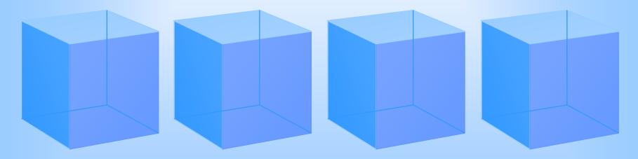
When the compressor squashes these four cubic metres to form one cubic metre there will be 4 times 8.7 grams, but only two of them can be held as a vapour in the new 1 cubic metre space. The other two have to condense out as water droplets
