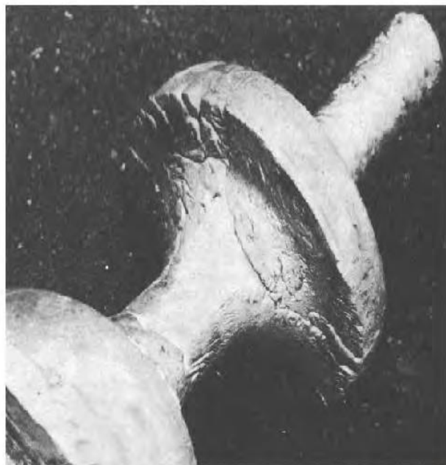
Figure 5.1 Cold laps and shut in a steel casting (courtesy of Institute of British Foundrymen)
