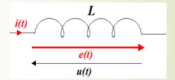
Where v(t) denotes the voltage in volts across the circuit and i(t) the current in amperes through the circuit.
