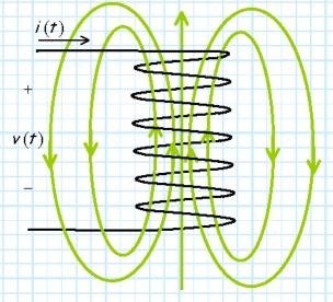
The current i(t) in flowing in the wire will produce a time-varying magnetic flux density within the solenoid. This time-varying magnetic flux density will **induce a voltage** v(t) across the solenoid.
