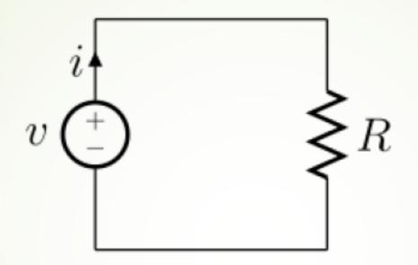
A simple electric **circuit**, where **current** is represented by the letter I. The relationship between the voltage (V), **resistance**(R), and current(I) is V=IR; this is known as Ohm's Law
